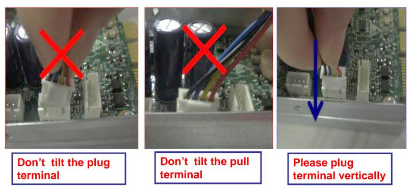
Improper plug and pull during wire assembly may affect conductor conductivity or fan performance, and cause no rotate problem.
