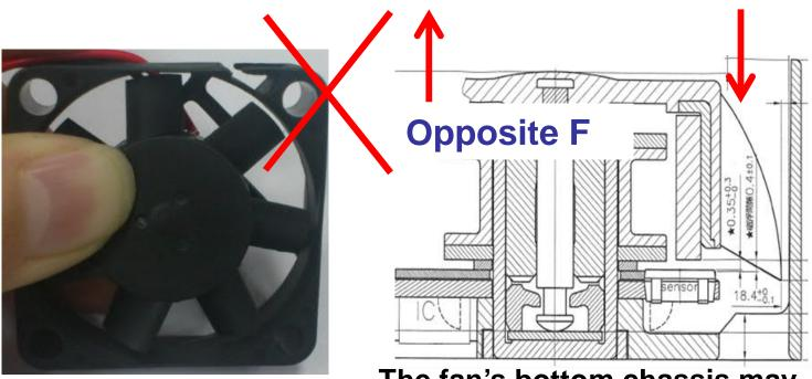
The fan's bottom chassis may deformation
