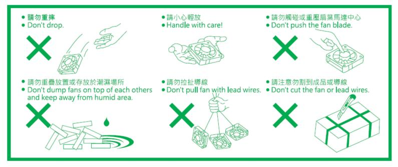
Don't dump fans on top of each others and keep away from humid area. Fans are at risk of falling off in a heap, which can lead to noise problem. Humid area will corrode the PCBA, and caused no rotate problem.
