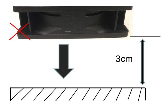
If the fan motor is dropped 3 cm away from the ground, it may damage the fan motors, and caused noise and vibration problem.
