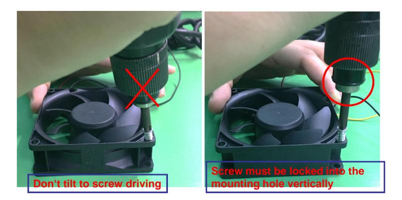
The frame is also a fragile part. In the assembly process, it should be noted that the screw must be locked into the screw hole vertically, otherwise there will be a risk of mounting hole facture.
