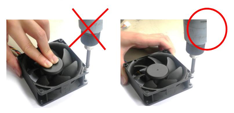
•When installation, please avoid to fix the fan by push the impeller, it may lead to the friction sheet sink. When friction sheet sink, its structure maybe changed. External forces will press on the ball bearing dust cap, and caused the fan noise problem.
