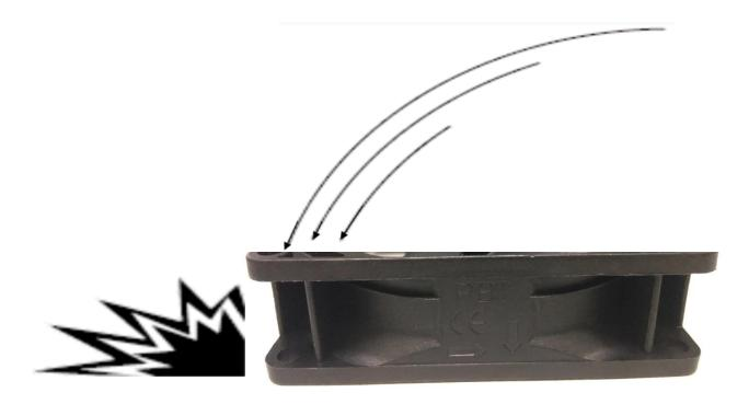
If the fan motor is knocked down from vertical to horizontal as shown in the picture, it depends on what material the floor is made of, but there is a possibility that it would damage the race surface of the bearing and it may cause the noise problem.
