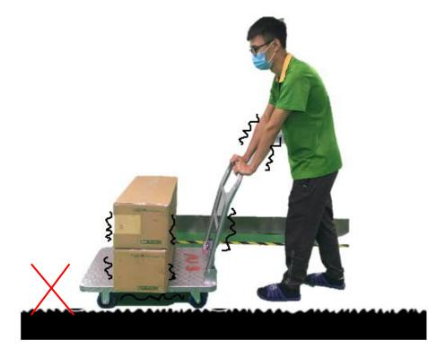
When transporting the fan motor with a hand truck, please avoid to go the bumpy road for a long time. If an excessive vibration is applied to the fan motor for a long time, it may damage the race surface of the bearing and cause noise problem.
