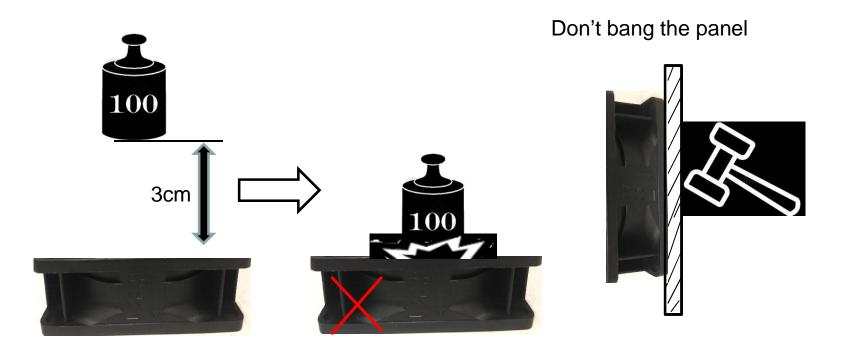
If an object that is 100 g is dropped 3 cm away from the fan motor, it may damage the fan motor, and caused noise and vibration problem.
